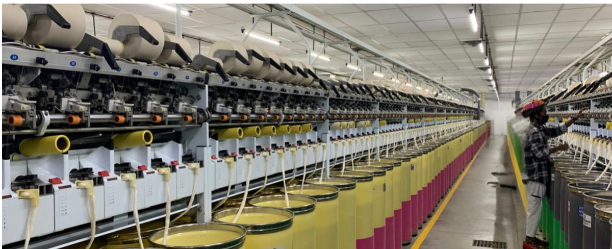
BD 480 rotor spinning line at Balaji Mill funded by GFF, replacing older BD 200 rotor line
